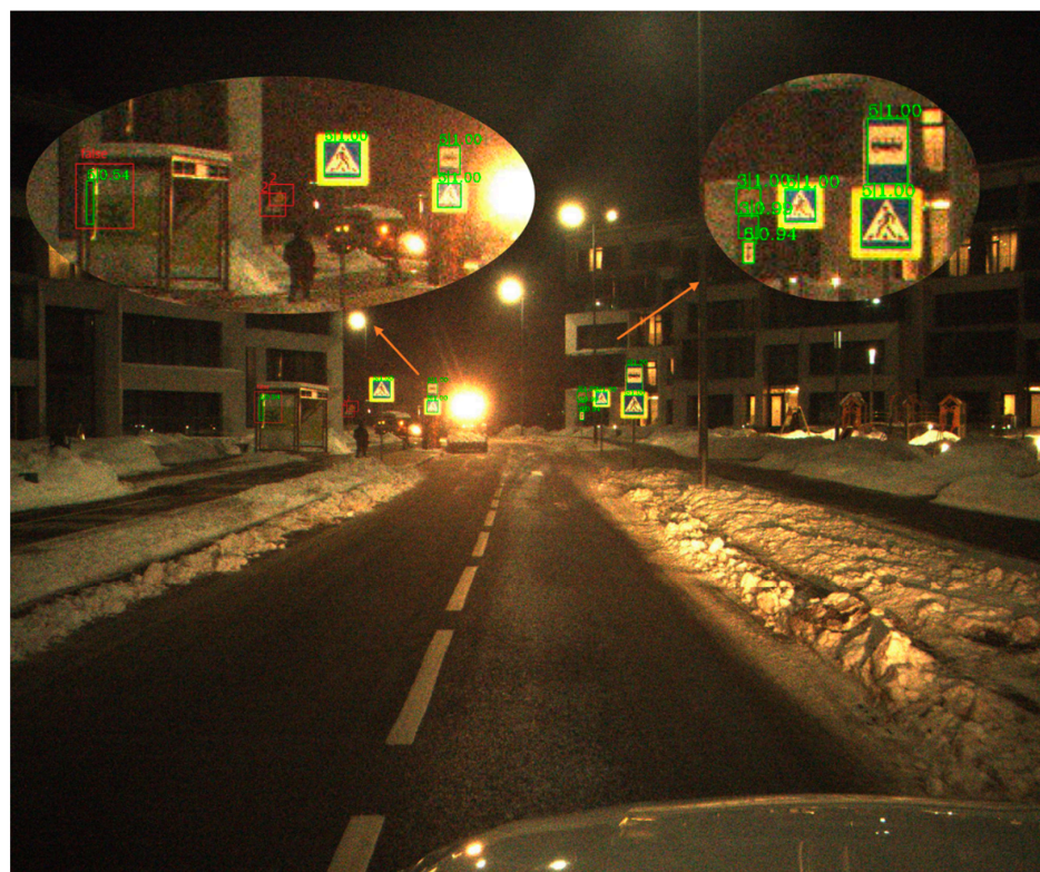
Figure 7. The visualization of the Faster-RCNN result on ITSDB detection. Green square represents detection result of the model, and red square represents target missed or detected wrong.
