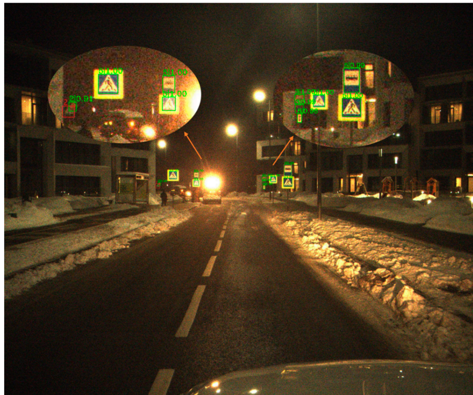
Figure 6. The visualization of the Libra-RCNN result on ITSDB detection. Green square represents detection result of the model, and red square represents target missed or wrong detection results.
