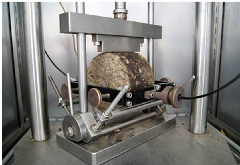
Figure 5. Scheme of the indirect tension test on cylindrical specimens (IT-CY) study.
