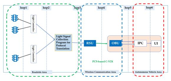
Figure 6. C-V2X SPAT Application System Architecture.
