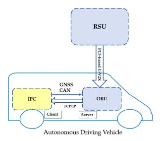
Figure 8. C-V2X Automated Driving System Integration.
