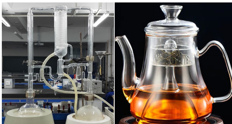
FIGURE 1 Similarity of simultaneous distillation-extraction (SDE) instillation (left) and tea cooking pot (right). Note: The temperature for SDE is the same as that for tea cooking. The SDE instillation and tea cooking pot have similar size in the outlet
