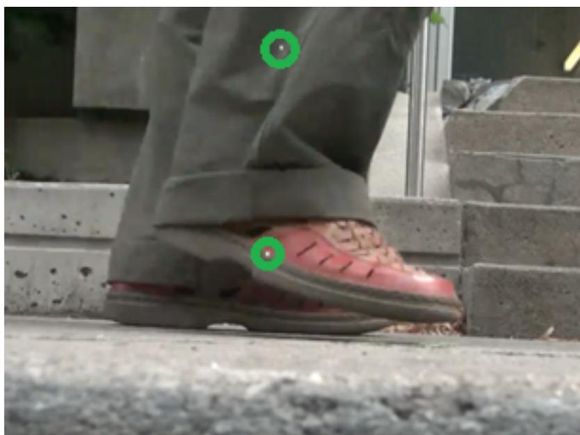
**Figure 4.** This image shows an example of a frame where the laser dots are projected onto the pedestrian's foot. The laser dots are marked with a green circle. The distance between the center of these two dots in the picture is equal to the fixed distance between the two laser pointers on the device.
