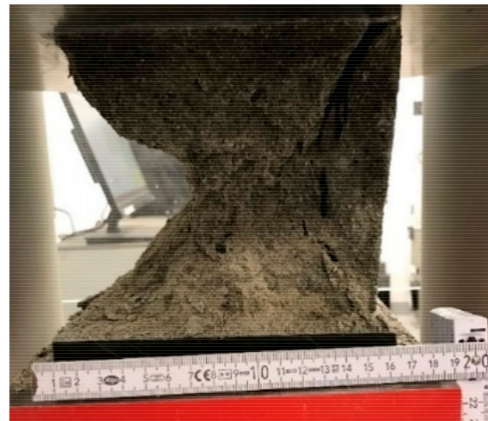
Figure 8. Destruction of sample with 1800 g/m 3 glass fiber addition in the compressive strength test.
