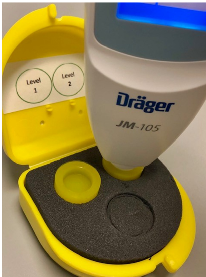
Fig. 1. Image of the in-house developed TcB QC material being measured using the Dräger Jaundice Meter 105®. The yellow material on the left is a Level 1 (L1) QC and its measurement corresponds to the low/medium risk (green/yellow zones) section of the locally validated TcB nomogram; yellow material on the right is a Level 2 (L2) QC and corresponds to the high risk (red zone) of the locally validated TcB nomogram. (For interpretation of the references to colour in this figure legend, the reader is referred to the Web version of this article.)
