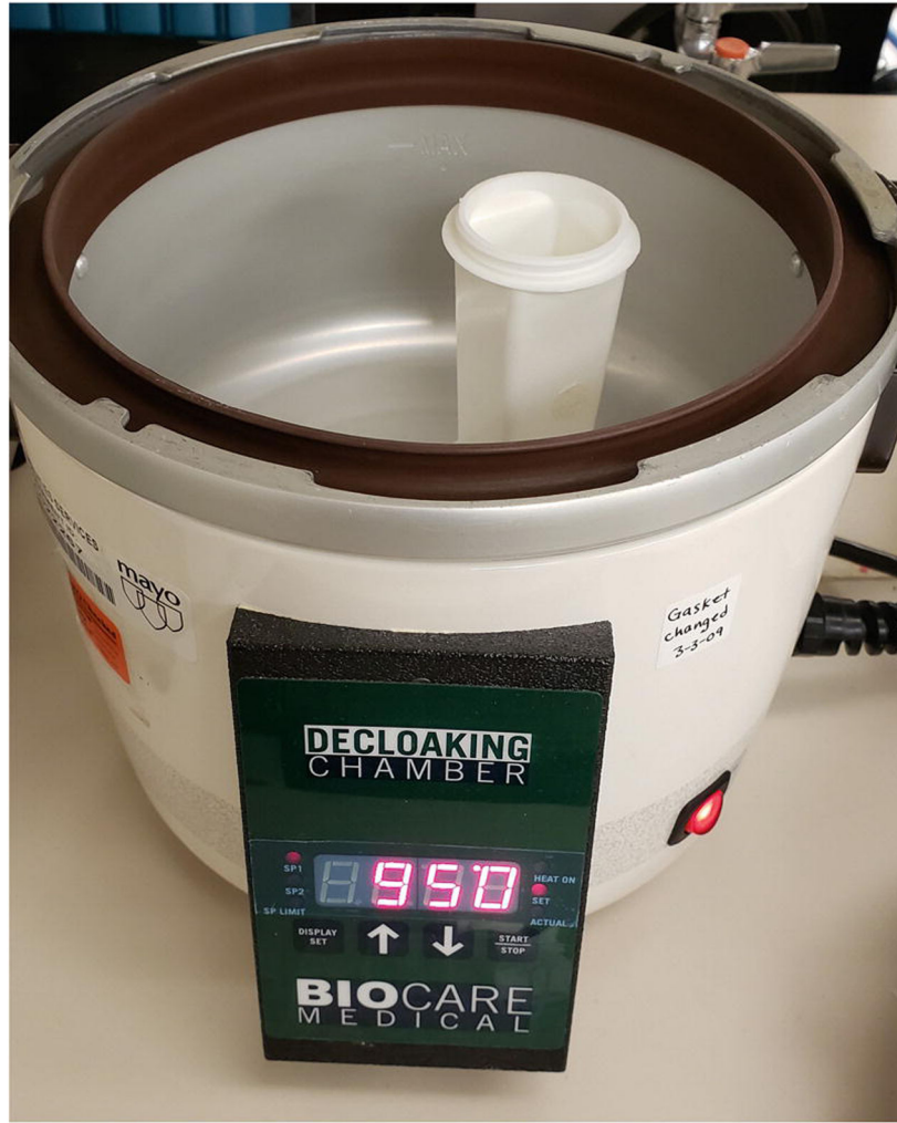
Fig. 3. Decloaking chamber (BioCare) with a plastic coplin jar. Water (500 mL) is placed inside the decloaker to distribute the heat around the coplin jar
