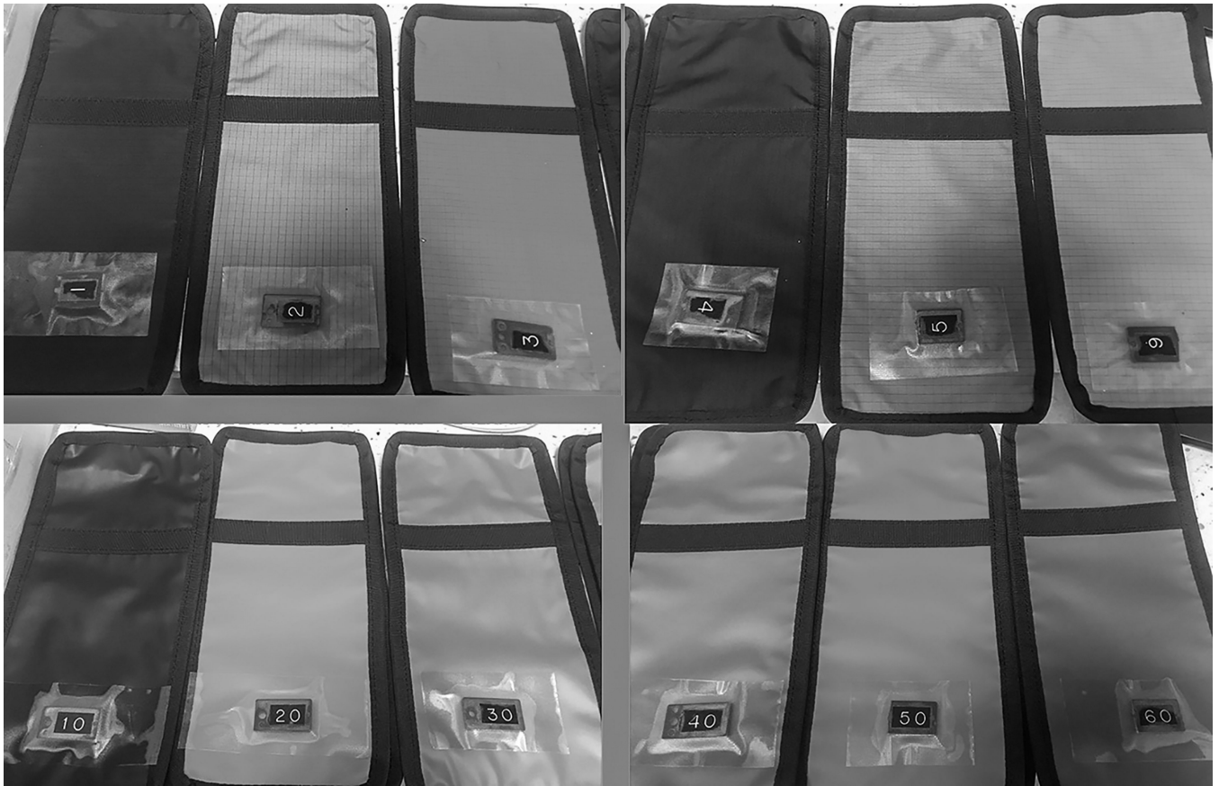
Figure 4). Final appearance Wipes A (left) and C (right) after 6 months of continuous contact with the cleaning agent.
