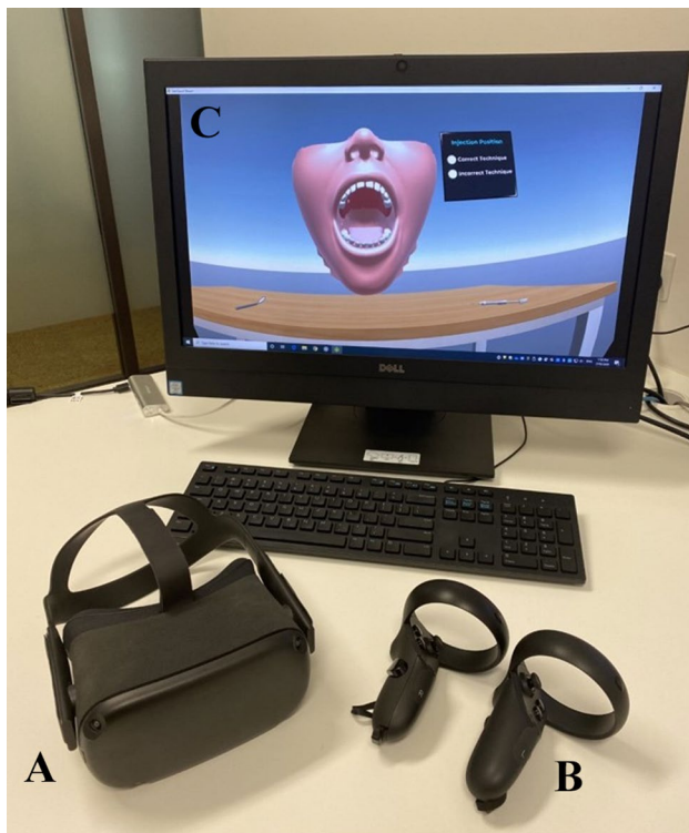
Fig. 1 Paediatric virtual reality local anaesthetic setup. a Oculus Quest headset b Hand controllers. c Stream function with SideQuest
