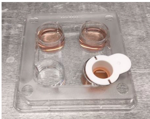
Fig. 2 PAFs are placed in a mini cell strainer immersed in cryoprotective agents (ES and VS) in a 4-well plate. Mini cell strainers are transferred with tweezers between different media and equally serve as cryo-container when they are plunged in LN 2
