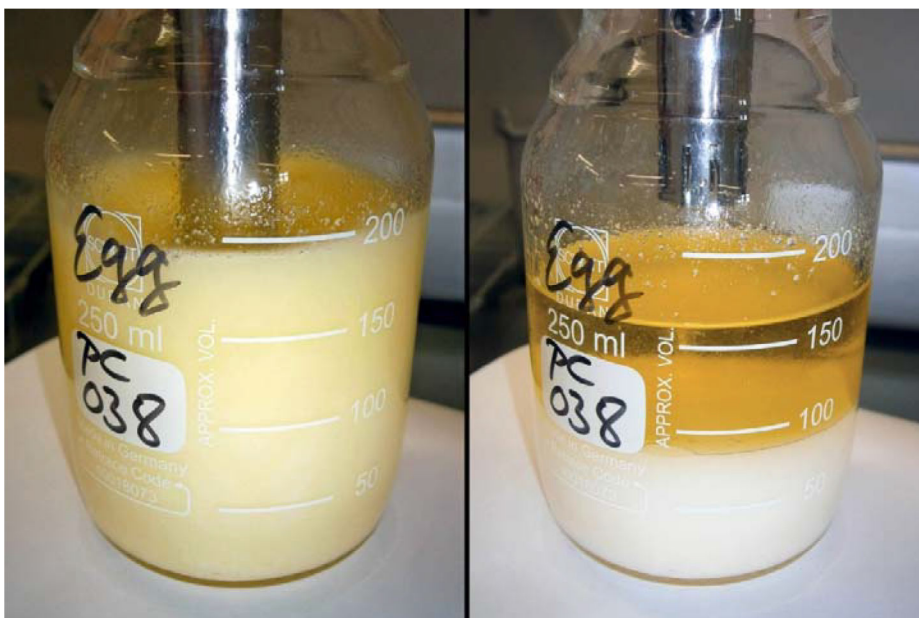
Figure 1. Modified Smedes extraction (MSE) of “total” lipids. Left: 15 s dispersion of 10 g chicken egg with 32 mL propan-2-ol, 40 mL cyclohexane and 24 mL water (“Ultra-Turrax B” in Table 2); right: 30 s after rinsing the rotor-stator with 5–10 mL propan-2-ol and brief circular swirling on a flat work surface. The clear upper organic phase was collected with a glass pipette connected to a pipette controller.
