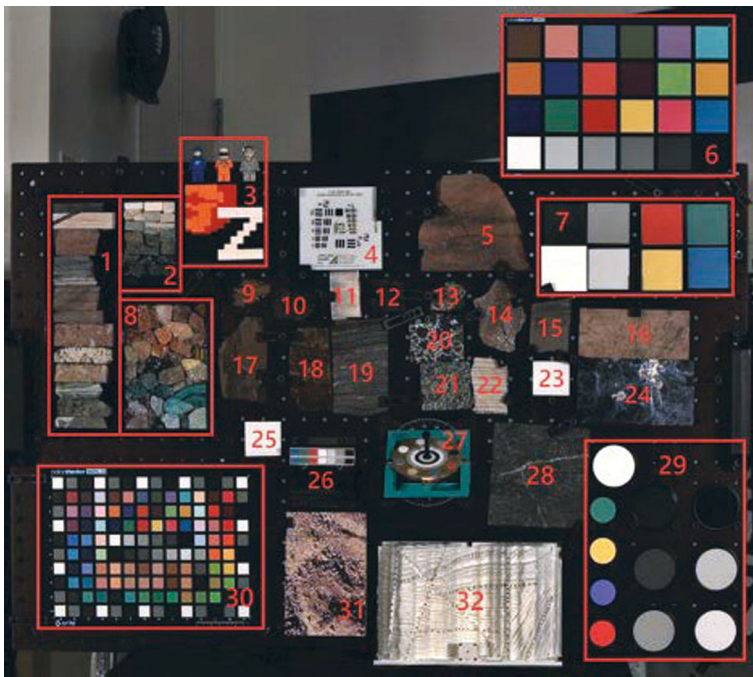
Fig. 38 The Mastcam-Z “Geoboard” imaged under ambient pressure and temperature conditions by Mastcam-Z (34 mm focal length, R0 filter, Bayer RGB color). Geoboard targets include color standards, rock slabs, resolution targets, stereo calibration targets, and education and public outreach materials. Target labels correspond to the names and descriptions provided in Table 11. For scale, the grid holes on the board have 1 inch spacing
