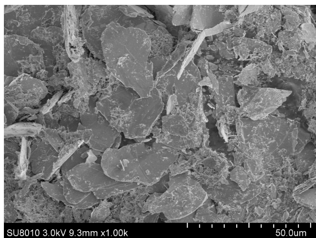
Fig. 6. FESEM micrograph of ultrasonic-assisted exfoliated NbSe 2 micro/nanoparticles after ageing for 15 days.
