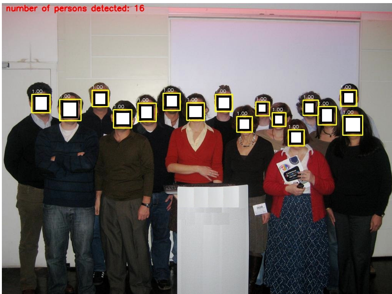
Figure 8. The output result of the proposed YOLOv3, which aimed to recognize a large number of persons (released from WIDER dataset [34]).
