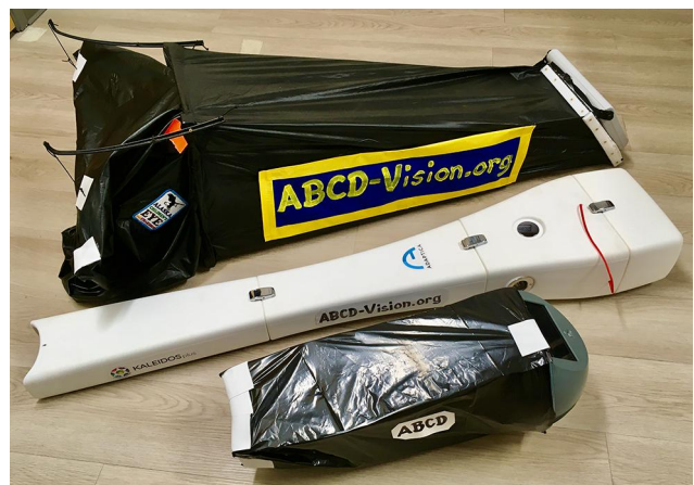
Figure 4 Three modified, portable amblyopia screeners, the Rebion blinq (foreground), the plusoptiX s12 (background) and the Adaptica 2WIN in Kaleidos case ready for outdoor, Drive-By photoscreening.
