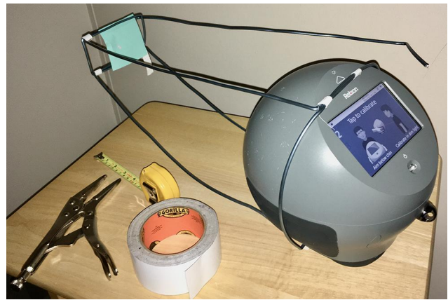
Figure 3 Wire-in-plastic frame to afford opaque covering for the Rebion blinq to be used outdoors.
