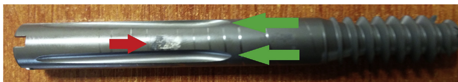
Fig. 2. Photograph from the removed lag screw. The red arrow shows the footprint of the malposition of the set screw outside of the grooves (green arrows). Each lag screw has four grooves, while the correct position of the set screw into the grooves allows lateral sliding and prevents rotation.
