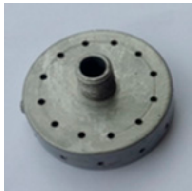
(c) Manufactured FFD with outlets holes at top and side
