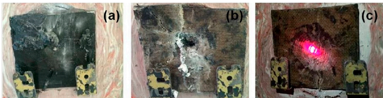
Figure 16. Images of jute fabric at (a) 10, (b) 20, and (c) 30 vol% as second layer in the multi-layered armour system (MAS) polyester composite. (Adapted with copyright permission from Monteiro et al. [117]).
