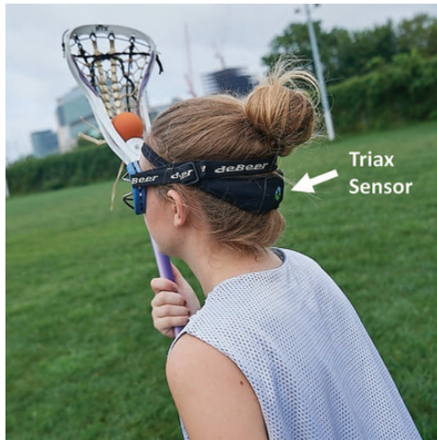
Figure 1. Lacrosse athlete wearing the Triax Smart Impact Monitor (Triax Technologies, Inc) headband-mounted sensor. Photo courtesy of Children’s Hospital of Philadelphia.
