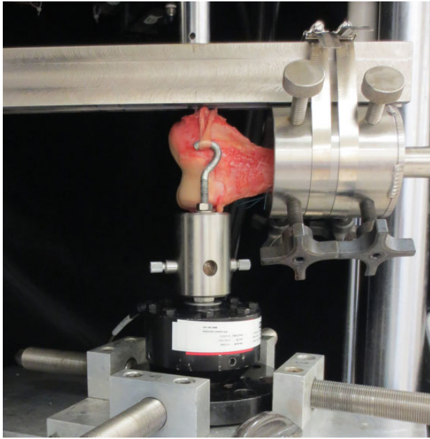
Figure 6. Biomechanical testing setup with the left femur secured to the MTS Mini Bionix load frame with the looped end of the 2-limb hamstring autograft attached to the load cell.
