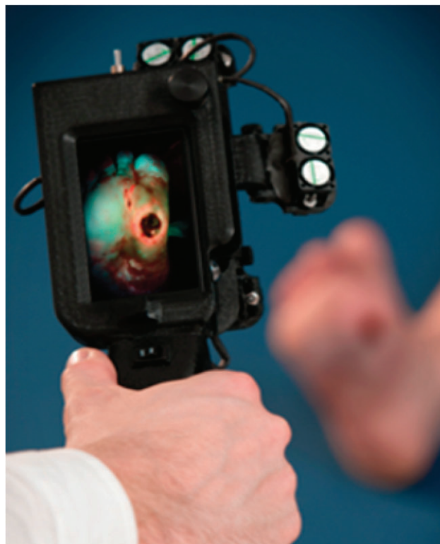
Figure 1 Photograph of PRODIGI device. The prototype handheld fluorescence imaging device aimed at a diabetic foot ulcer. Fluorescence images are displayed in real time on the colour liquid crystal display (LCD) touch screen. Dual broadband white light and violet light emitting diode (LED) arrays provide illumination of the wound, while the autofluorescence signals from the wound and surrounding healthy tissues are detected by the device's complementary metal-oxide-semiconductor (CMOS) image sensor in real time.
