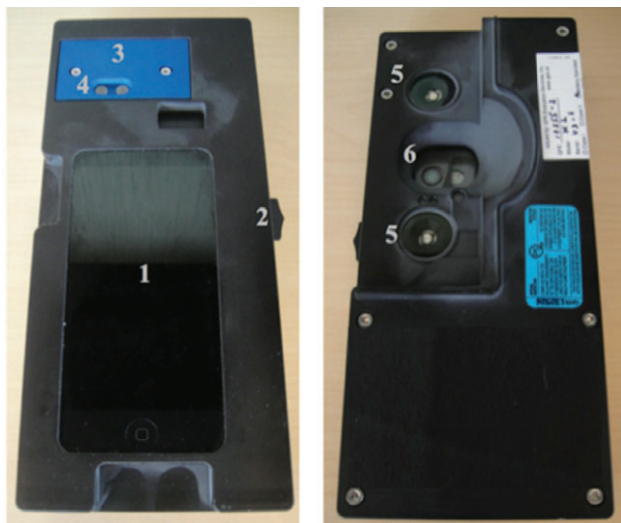
Figure 1 The prototype K2 imaging device used in the study. The front view (left) shows (1) the integrated iPod camera, home button and display screen built into the device housing, (2) the sliding light emitting diodes (LED)-activation mechanism, (3) the heat sink to safely dissipate LED heat, (4) the range finder and ambient light LED indicators. The back view (right) shows (5) the two 405-nm emitting LEDs, (6) the imaging detector and sliding emission filter and labels for device identification and certification.
