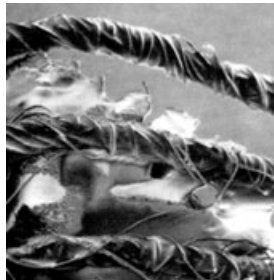
Figure 2. Structure of TG showing unraveling and dislodgment of gauze threads.
