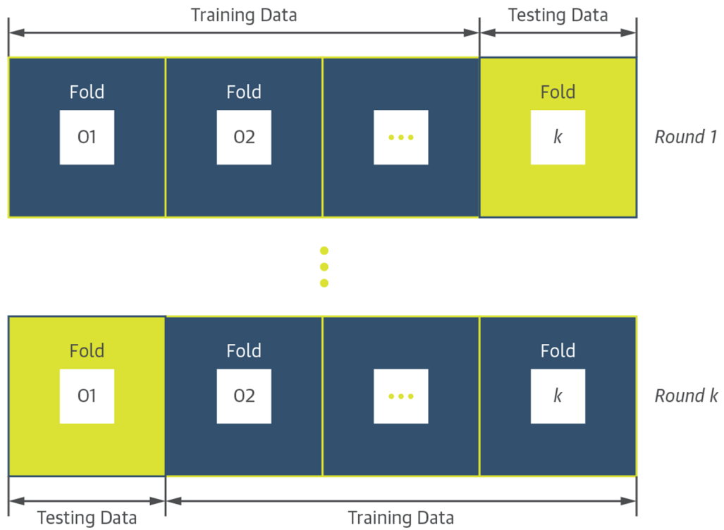
FIGURE 5. Schematic Illustration of the K-Fold Cross-Validation Process
