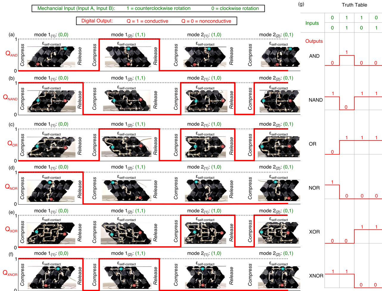
Fig. 5 Processing all digital logic operations in soft, conductive mechanical metamaterials. Logic gate digital output Boolean response at each of the four compact states for the (a) AND, (b) NAND, (c) OR, (d) NOR, (e) XOR, and (f) XNOR logic gate. The respective mechanical inputs (green) for each of the deformation states directly relate to (g) the logic gates truth table inputs.
