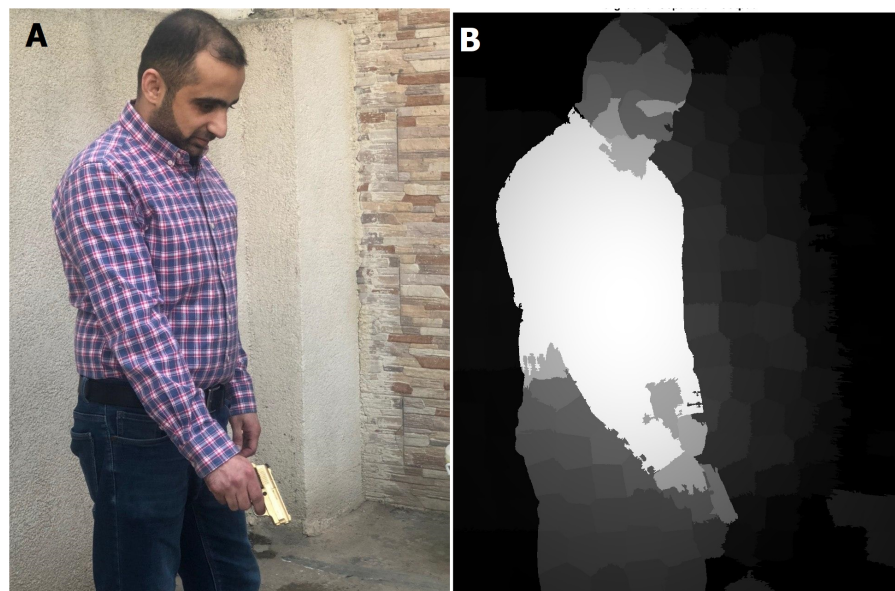
Figure 8 Saliency map results for humans with a gun (in real time streaming). (A) Streamed images; (B) the output (saliency results) of streamed image (A).
