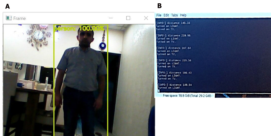
Figure 10 Detection process of the proposed system. (A) Human detection screen, a green square represents the detected human. (B) Human distance calculation (the system computes the distance of the human from a wall when entering the surveillance area and activates the light (light text in figure) at distance of 5 meter and making alarm with showing the camera view in monitor screen where human detect (TV text in figure).
