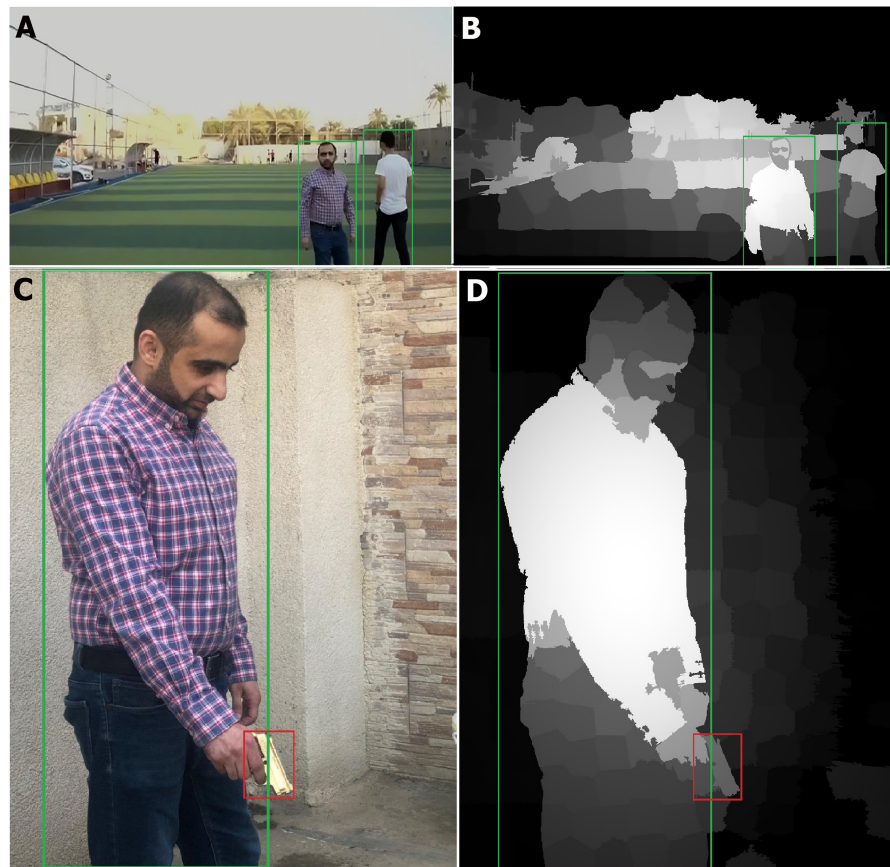
Figure 9 Detection results (in real time streaming). (A) Detection of two humans in the sense; (B) sense output for humans detection; (C) detection of human with gun; (D) sense output for humans and gun detection.
