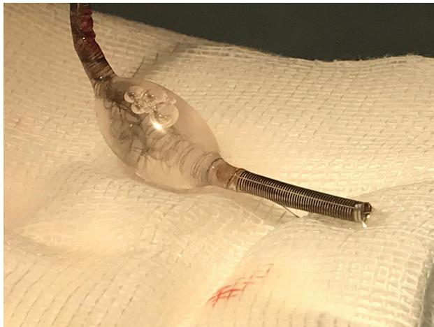
FIG 1. The JET 7 catheter used in the thrombectomy for patient 1 shows ballooning of its distal end with separation of the reinforcing braids from the surrounding polymer.
