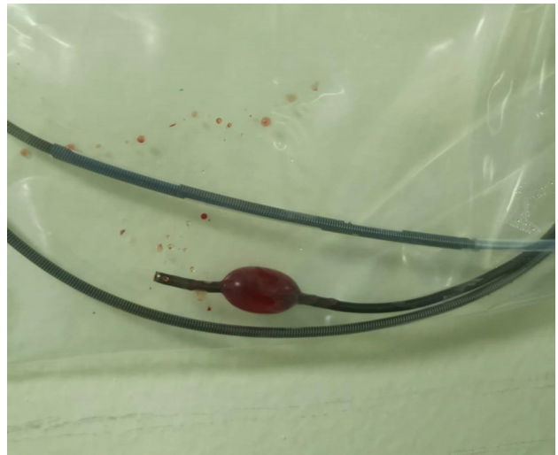
FIG 2. The damaged distal segment of the JET 7 thrombectomy catheter used in patient 2 has ballooned on flushing.
