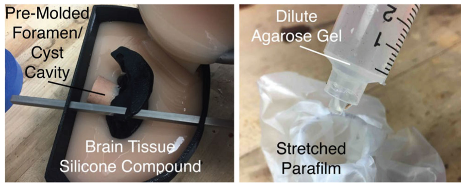
Fig. 8: (Left) The brain tissue silicone mold is poured with the ventricles assembled using the square rods, and the foramen/cyst cavity already pre-cast out of stiffer silicone. (Right) Cyst preparation: the stretched Parafilm is placed over a tube and a syringe is filled with dilute agarose gel mixture.
