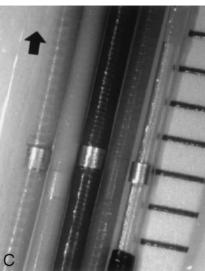
Fig 2. Photographs and fluoroscopic images show proximal and distal catheter markers, catheter part extended from distal catheter marker (real end of microcatheter), and distance between catheter markers. The diameter of the *black circle* in the fluoroscopic image is 1 cm. A division of the ruler shown in the photographs (*A* and *C*) is 1 mm.
