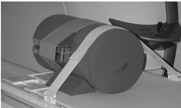
Fig 3. The 18 samples of the programmable valve shown attached to the cylinder-shaped phantom in preparation for the static magnetic field exposures (sagittal orientation).
