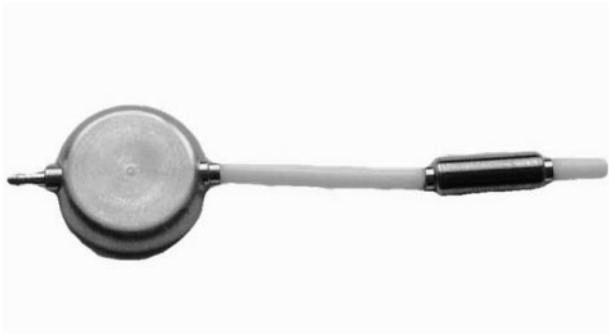
Fig 1. The programmable valve that underwent evaluation for MR imaging safety at 3T. The nearest 1° was measured 3 times, and an average value was calculated. 11-15
