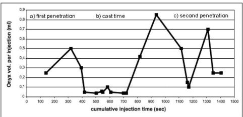
Fig 2. Typical injection curve of one feeder treated with 4.77 mL Onyx (feeder 4 from Table 2) demonstrating the typical injection phases: A, first penetration (<400 seconds); B, cast time or precipitation time (400–700 seconds); and C, second penetration (>700 seconds).
