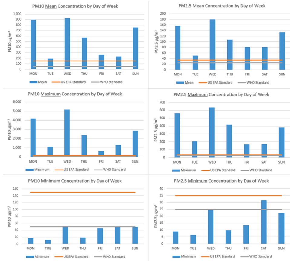
Fig. 2. PM 10 and PM 2.5 field test results. Note: Two straight lines in each graph are US EPA & WHO standards.
