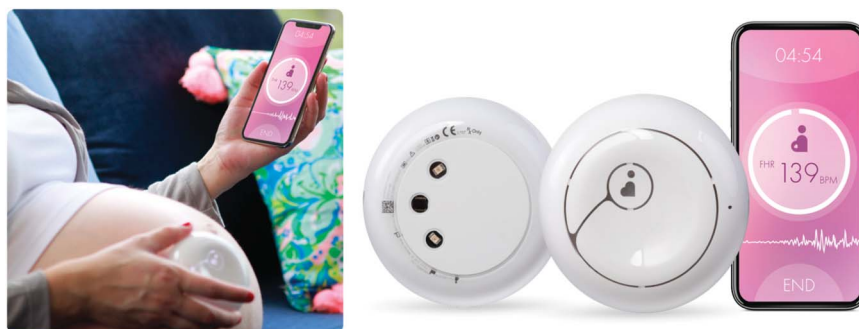
Fig. 1. Fetal heart rate monitoring system with the device and integrated smartphone interface. Image courtesy of HeraMED Ltd. Used with permission.
