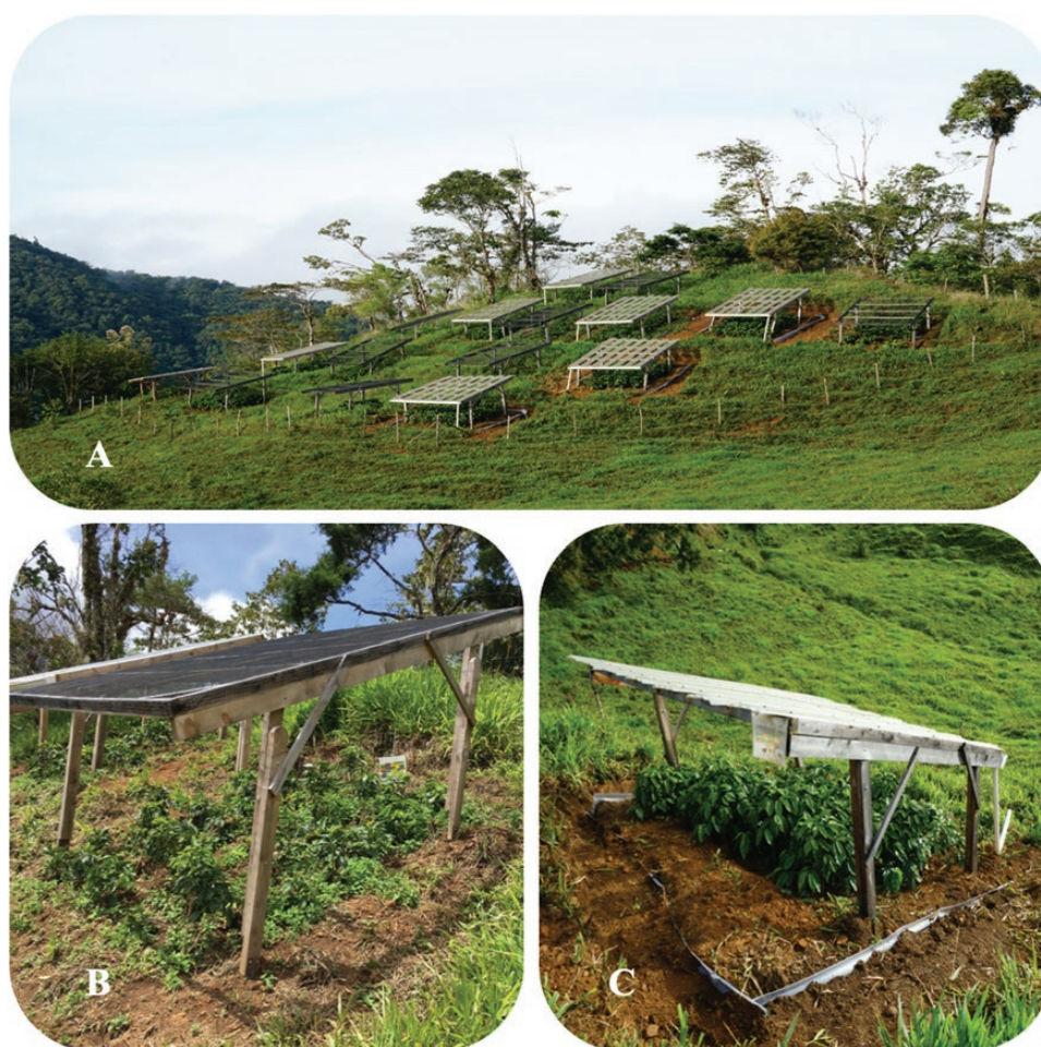
Figure 2. (A) The research site near Santa Maria de Dota. (B) Control shelter with mesh roofing and (C) rainout shelter with polycarbonate roofing, gutter, pipes and in-ground plastic barrier.
