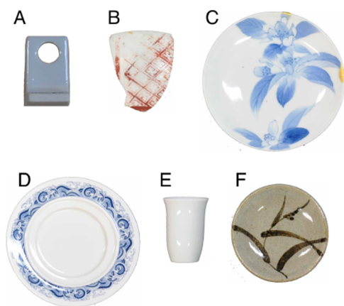
Figure 1. Analyzed glazed porcelain samples. (A) A test sample coated with a wollastonite glaze. (B) An ancient porcelain shard produced in Arita, Japan between 1650 and 1670. (C–F) Commercially available porcelains produced at (C) Seto, Japan, (D) Jingdezhen, China, (E) Meissen, Germany, and (F) Karatsu, Japan.
