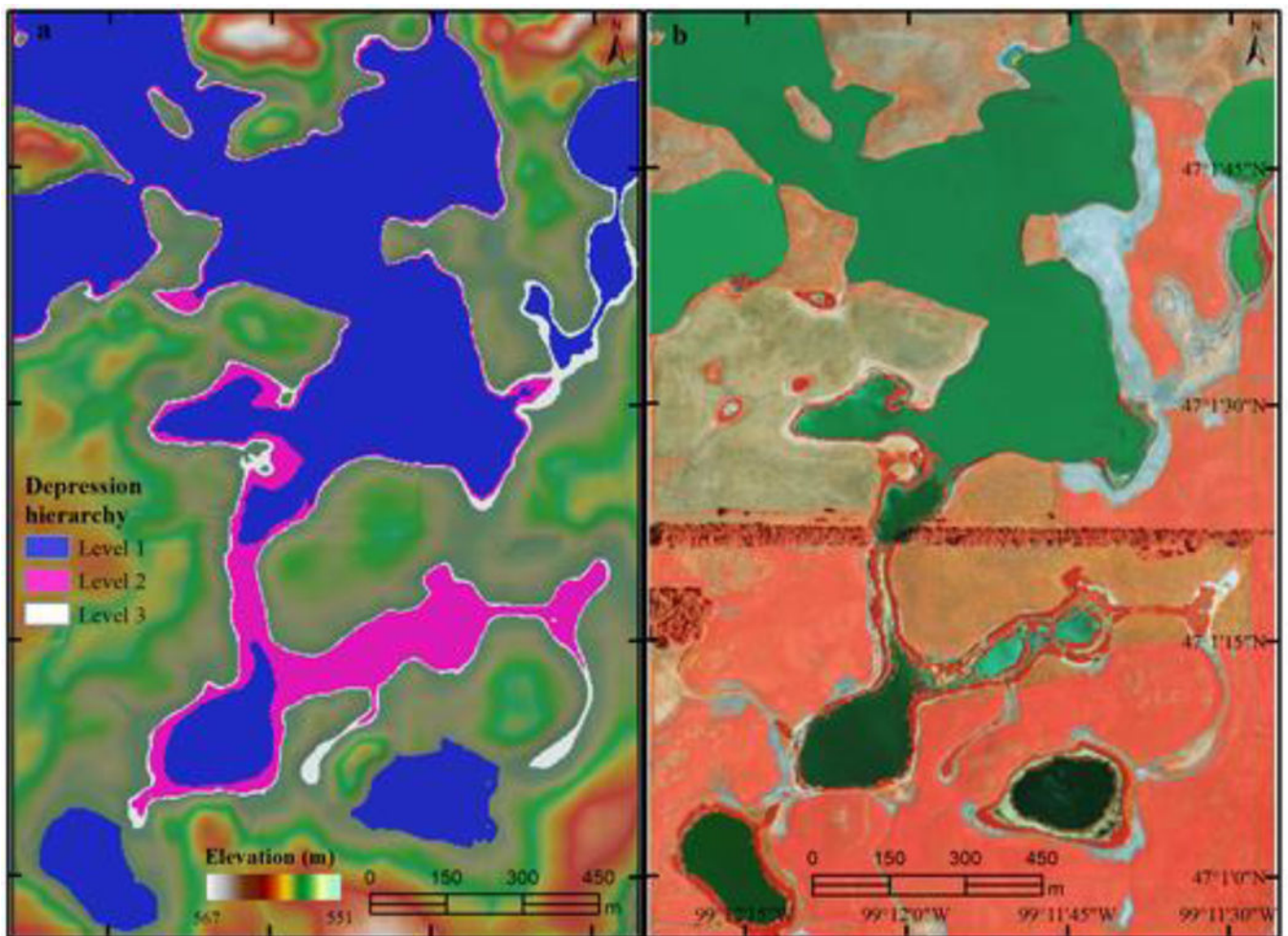
Figure 7. Sample area marked by the pink rectangle in Figure 6. (a) Nested depressions overlaid on the shaded relief map. (b) Four-band (RGBN) aerial photograph acquired on July 31, 2012.
