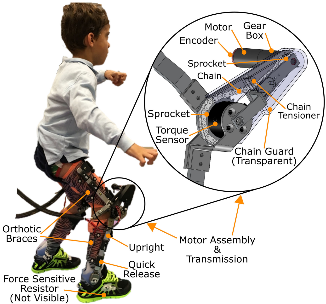
Fig. 1. Photograph and schematic of the robotic exoskeleton for knee extension assist to alleviate crouch gait from cerebral palsy.
