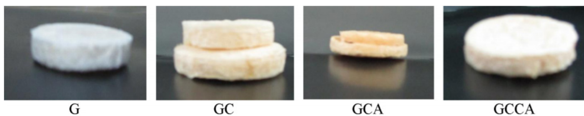
Figure 2. Different types of fish skin gelatin scaffolds. G: simple gelatin; GC: gelatin + chitosan; GCA: gelatin + calcium acetate; GCCA: gelatin + chitosan + calcium acetate [63].
