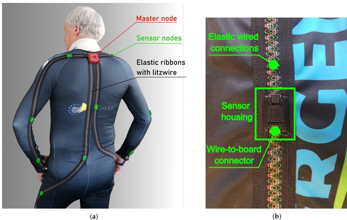
Figure 8. Experimental setup. (a) The sensor clothing with multi-branch IMU sensor network. (b) The custom 3D-printed housing used for sensor placement.
