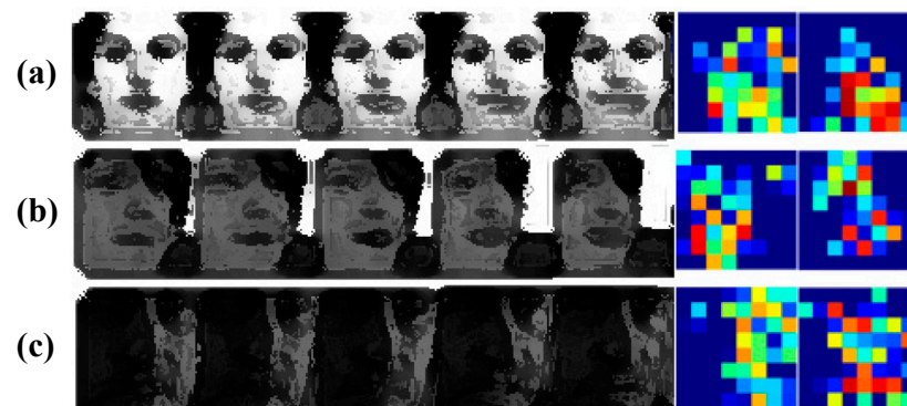
Figure 5. Visualization of hybrid attention module output features (weight increases from blue to red: dark blue–light blue correspond to 0.1–0.4, light blue–yellow correspond to 0.4–0.7, yellow–red correspond to 0.7–1). In the first five columns, the subfigures (a–c) show image sequences under (i) the ideal condition, (ii) the facial deflection condition, and (iii) the uneven illumination condition. We note that the resolution of the images in these five columns is reduced to protect the privacy. Those images are plotted with the purpose of displaying the profiles of eyes, nose, and mouth, which vary with facial expression changes generally. In addition, the second last column and the last column visualize the attention weights with self-attention and hybrid attention, respectively.
