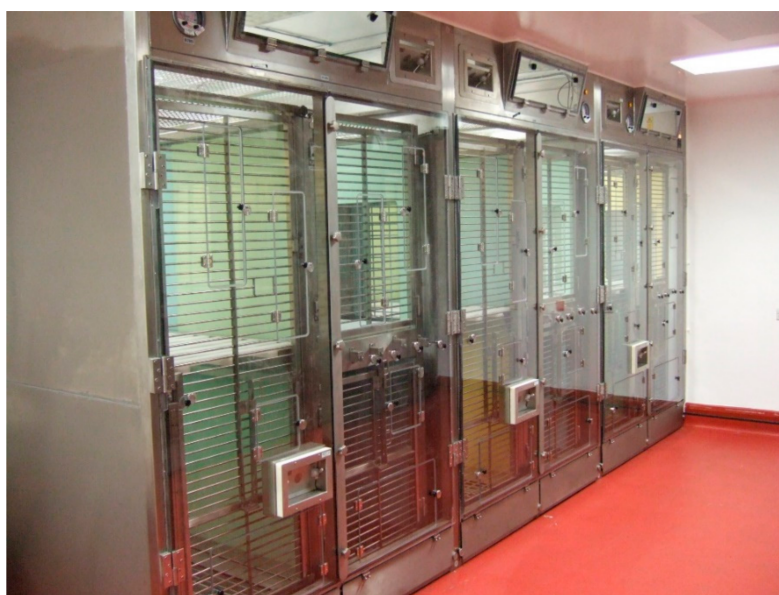
Figure 1. Containment system for group housing of macaques at Public Health England (PHE). Three cages are shown, each consisting of four units. (Image: Mike Dennis, PHE).
