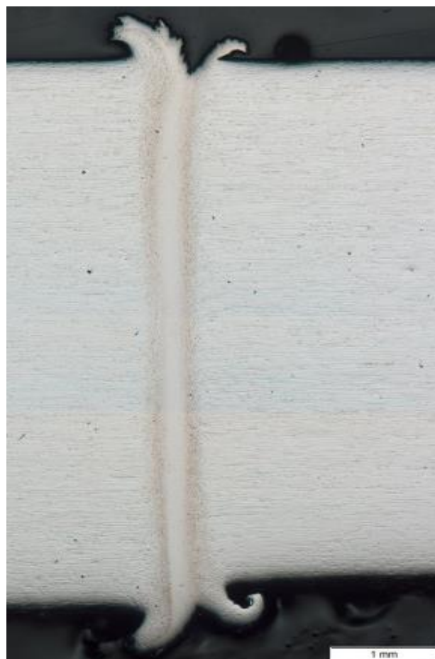
Figure 3. Macrostructure of the friction-welded joint from 316L steel after HE.
