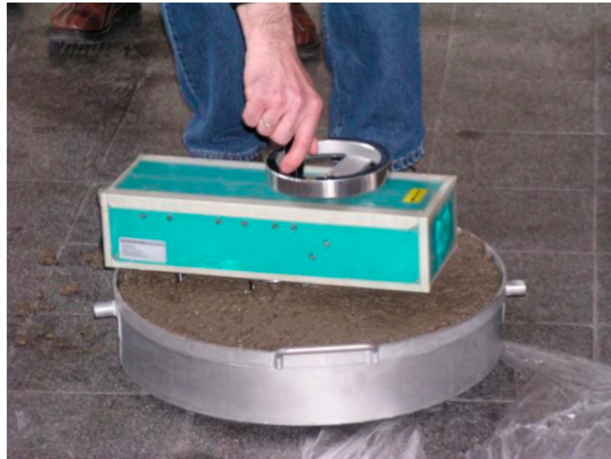
Figure 1. BT2 rheometer in use for the rheological properties determination.
