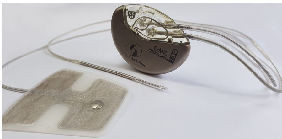
Figure 1 Implantable device with its left ventricular patch and right ventricular coil leads.
