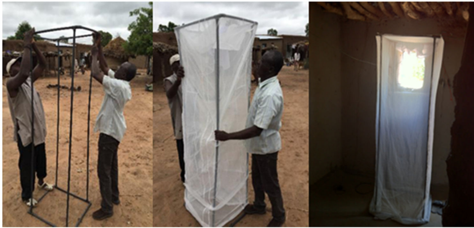
Figure 2: Field technician and local guide mounting an entry window trap
