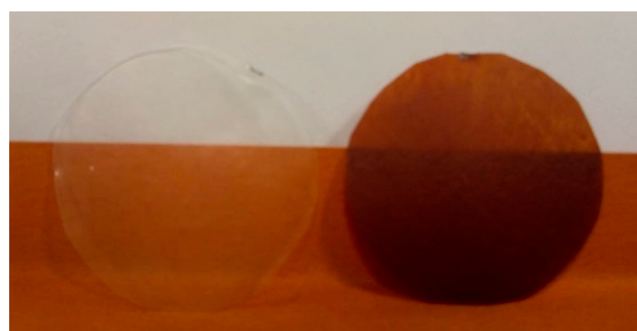
Figure 4. Digital photo of solvent-cast neat PLA film (left) and PLA film containing 10% w/w PNSE (right).
