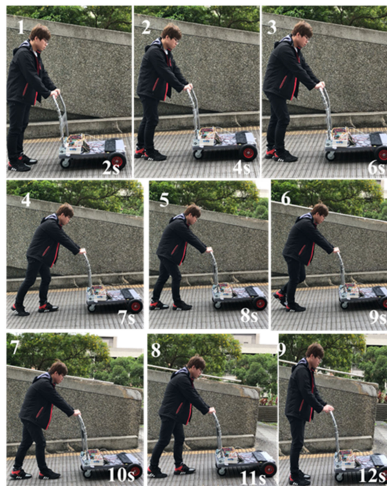
Figure 15. Snapshots of smart walker assisted on a steep uphill.
