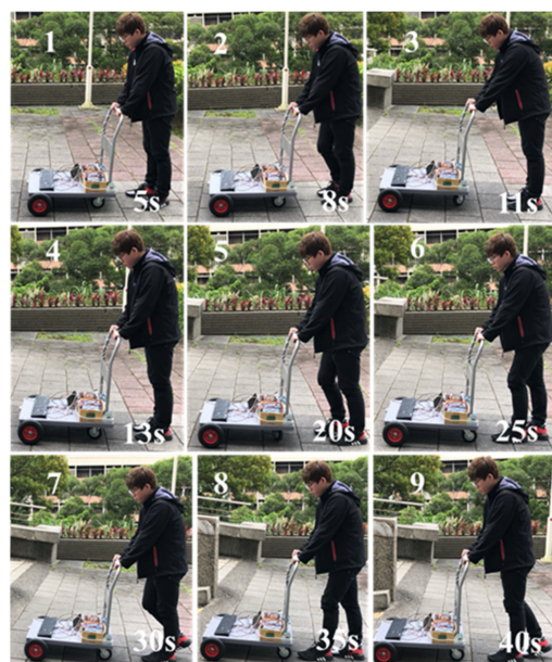
Figure 13. Snapshots of smart walker assisted in flat surface.
