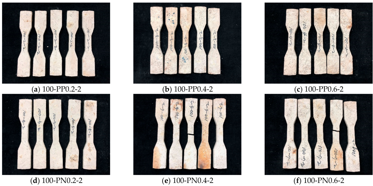
Figure A1. Appearance of the 100 MPa specimens after 2 h of fire exposure.
