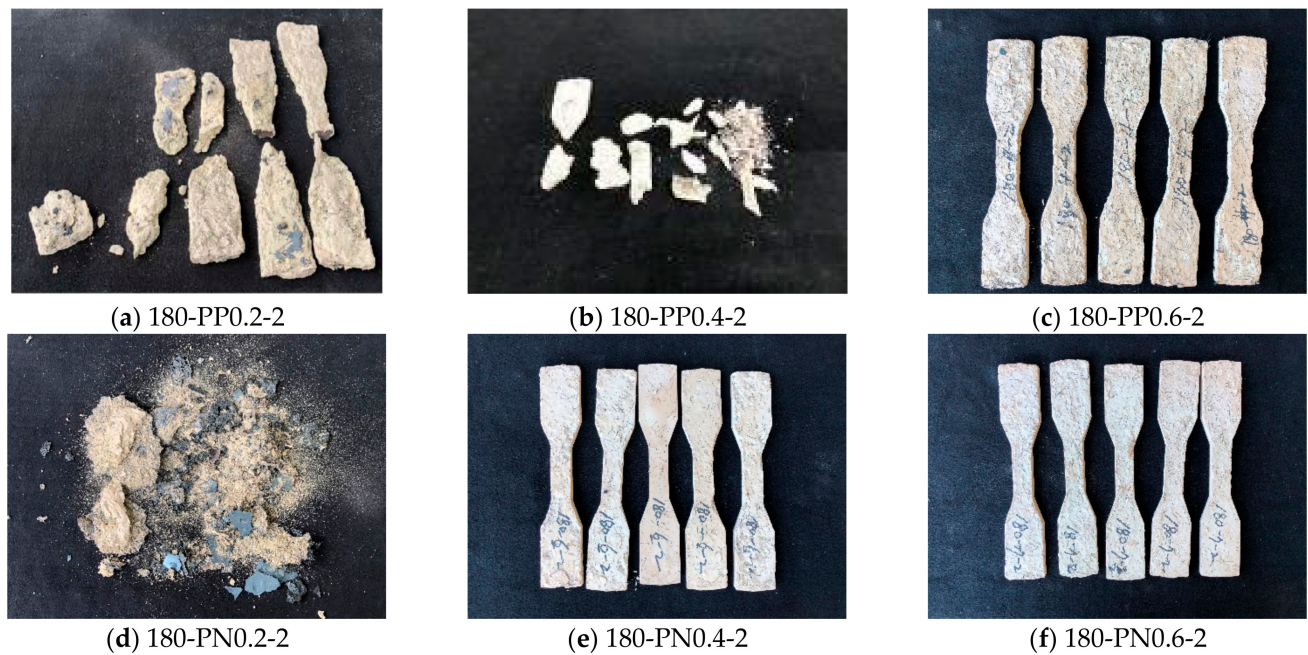
Figure 4. Appearance of the 180 MPa specimens after 2 h of fire exposure.
