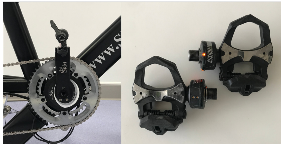
Figure 1. Representative example of the setting used on this study, placing the Favero Assioma Duo pedal power meter on an SRM crank.
